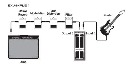
One use of the Vertex Volume/EXP Pedal is to place it immediately after your guitar. This is ideal for players that wish to have their volume pedal mimic the function of a guitar volume potentiometer, simultaneously cleaning-up the signal while reducing the output level, regardless of the effects placed after it (controlling the overall amount of gain).
