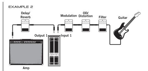
A second use of the Vertex Volume/EXP Pedal is to place it after filter, distortion, overdrive, and modulation pedals, but before any time-based effects. This is ideal for players that wish to attenuate the output level of their signal (master volume), while maintaining the same quality of the filtering, overdrive, distortion, modulation, and time-based effect trails without changing the tone.
